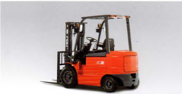
48V AC 4-Wheel Electric forklift CPD10-25 2000-5000 lbs.
