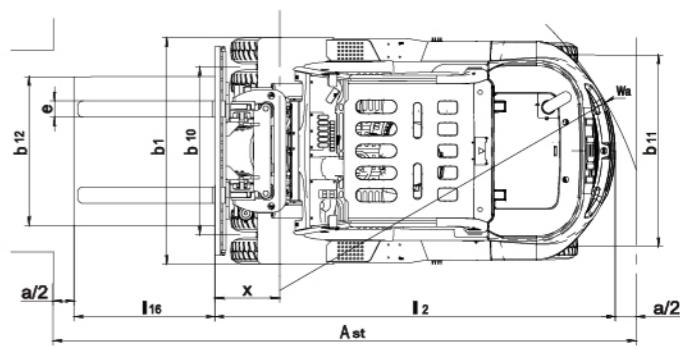
Ast: Right angle stacking aisle width
