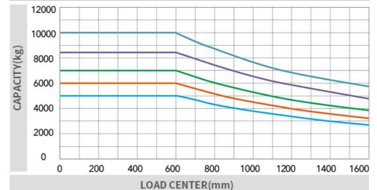
**Note:** The vertical axis stands for load capacity and the horizontal axis stands for load center which is calculated from the front surface of the forks to the gravity of the standard load. The standard load means a cubic with 1000mm edge length. When mast is tilted forward, using non-standard forks or loading large goods, the load capacity will be reduced. The load capacity of standard mast at different load center can be known from this load chart.
