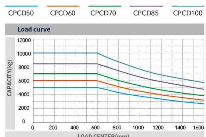
**Note:** The vertical axis stands for load capacity and the horizontal axis stands for load center which is calculated from the front surface of the forks to the gravity of the standard load. the standard load means a cubic with 1000mm edge length. When mast is tilted forward, using non-standard forks or loading large goods, the load capacity will be reduced. The load capacity of standard mast at different load center can be known from this load chart.
